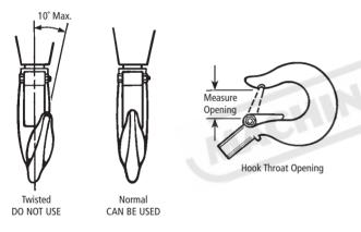
Any hook that is twisted or has excessive throat opening, indicates abuse or over loading of the unit. Other load sustaining components of the chain block should be inspected for damage. The chart above should be used to determine when the hook must be replaced. To measure throat opening, depress the latch against the hook body as shown above.
