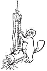
**DO NOT** shock load chain block, chain or hook.
