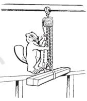
**DO NOT** hold the load chain in a loaded state while operating the chain block as serious injury may occur if the brake did not operate properly.
