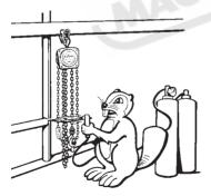
**DO NOT** heat treat and DO NOT weld any part of the chain block, expecially the load chain.
